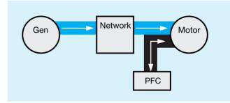
The inductive reactive power  $Q_1$  is compensated for totally or partially by the capacitive reactive power  $Q_{\text{comp}},$  the apparent power thus being reduced from  $S_1$  to  $S_2.$
