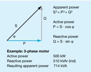
Although the motor's mechanical power output only calls for 500 kW, the supply network loading is an apparent power of 714 kVA, i.e. it has to transmit 143% of the active power.
