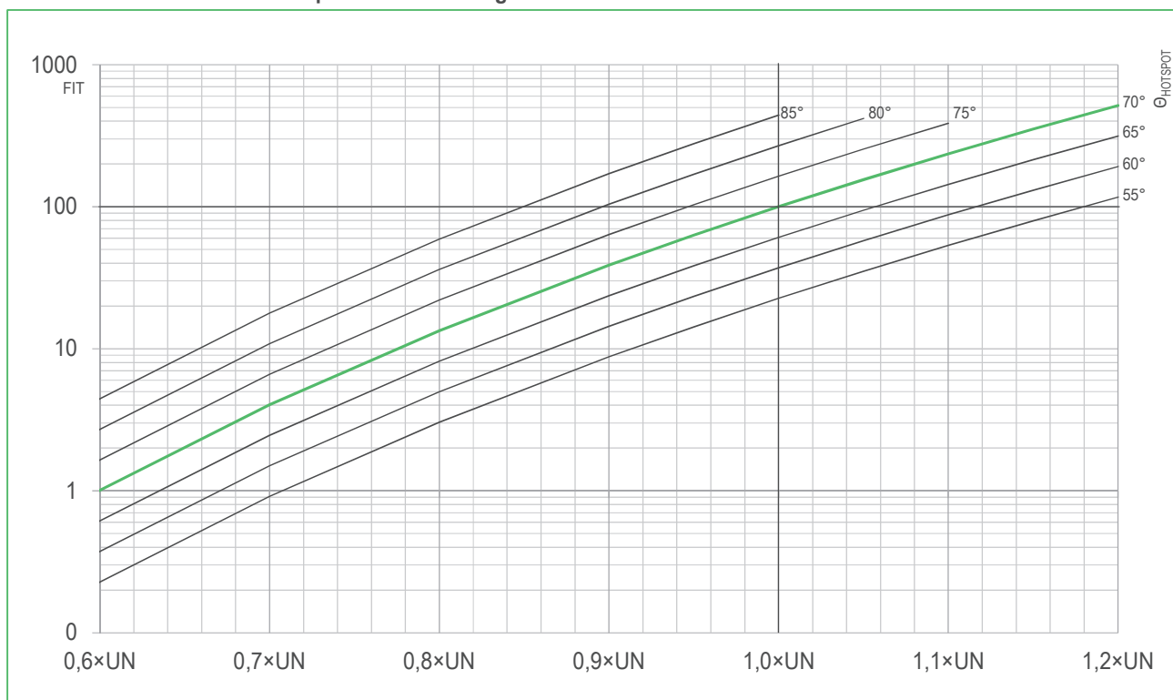
FIT-RATE versus HOTSPOT temperature and voltage
